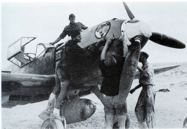
LEFT: Ground personnel fastening the engine cowling on 'White 5', the Bf 109 E-7 Trop flown by Lt. Werner Schroer of 1./JG 27. The camouflage on the fuselage of this aircraft was in the form of a continuous wavy line, which later became known as the Wellenmuster, or wave-type, camouflage.
