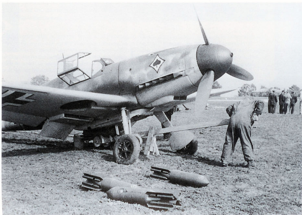
ABOVE: In a deliberate attempt to enhance the terror effect of falling bombs, cardboard whistles were sometimes attached to the tail fins, as seen in this view showing Uffz. Felix Sauer of 10.(Jabo)/JG 53 at Gela in April 1942.
