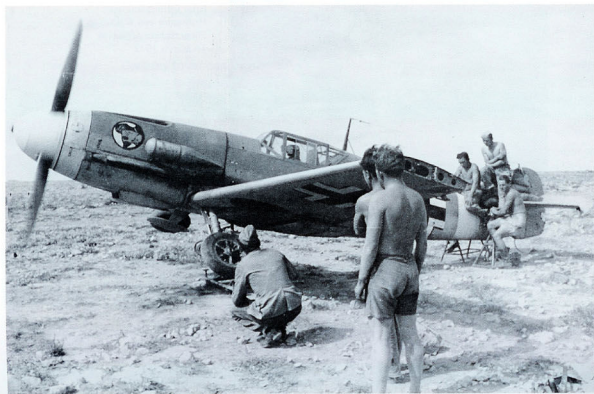
LEFT: Jacked up on trestles, a Bf 109 F undergoes undercarriage retraction tests, but a new wingtip will be required before the aircraft can be signed off as fully airworthy. In order to ensure that the machine does not nose over, sandbags have been placed on the horizontal tail surfaces and a number of ground crew provide added weight.
