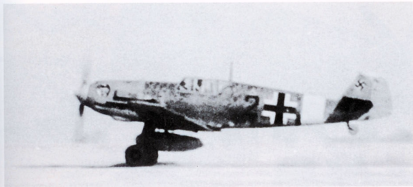
ABOVE: Desert sand was highly abrasive and aircraft paintwork quickly weathered, as may be seen on the spinner and lower engine cowling of this Bf 109 E from 1./JG 27 which was photographed while being repainted.
