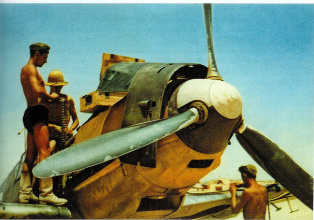
LEFT: Armourers re-loading the fuselage-mounted MG 17 machine-guns on a Bf 109 E of JG 27. Although unquestionably taken in the Western Desert, this photograph clearly shows the grey and green camouflage and conspicuous yellow tactical nose markings previously employed in Europe.
