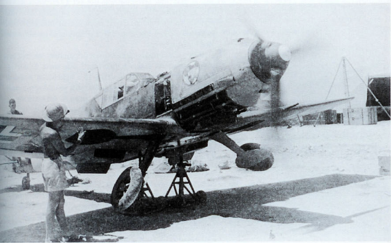
THIS PAGE: A series of photographs showing 'Yellow 7' of 3./JG 27 during undercarriage retraction tests in North Africa.
